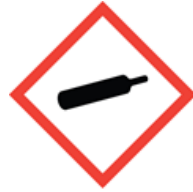
Gas Under Pressure
